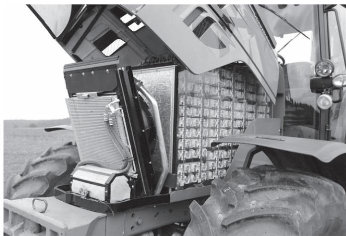
**In 2017, John Deere showcased the first fully battery-powered tractor. This technological innovation is truly the first of its kind. Nicknamed SESAM, for Sustainable Energy Supply for Agricultural Machinery, this all-electric tractor is modeled after John Deere's 6R series tractors.**
